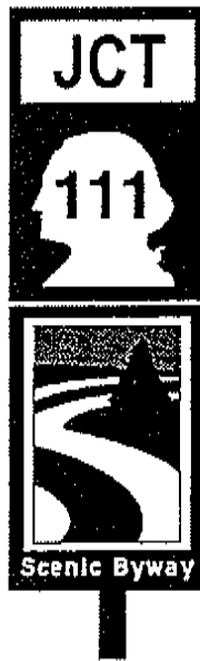
Example of combined scenic byway logo sign and route marker on single signpost from WSDOT Scenic Byway Logo Signing Guidelines
